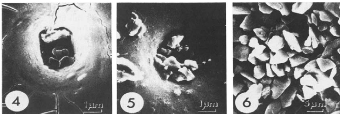
Fig. 4. The same diaphragm observed after several hours of use. Solvent, acetonitrile-water; stationary phase, LiChrosorb RP-18 ( 5\ \mu\text{m} ).
